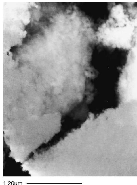
Fig. 7. SEM image of chromia-based catalyst treated with HF at 140 °C.
